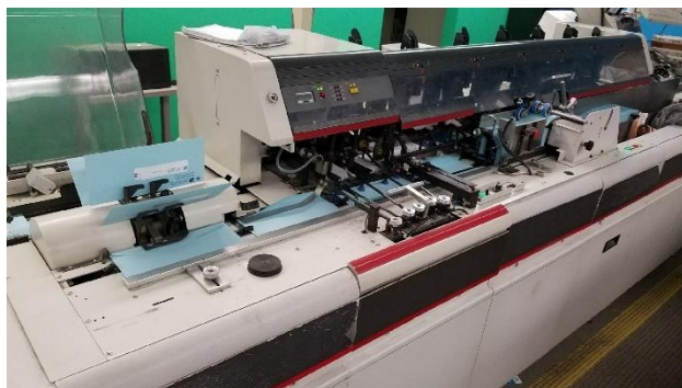
Mail Inserting Machine (used to insert bills/notices, etc. into envelopes and affix postage).
