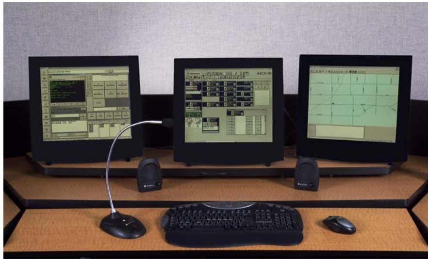
Figure 3-1: Typical layout of the MCC 7500 console in a dispatch center along with two other public safety terminals.
