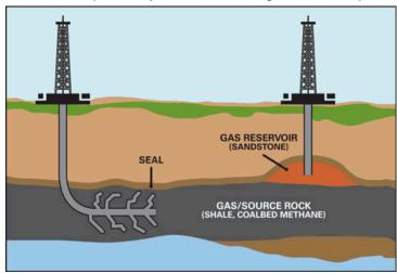
accessing this gas. The method is quite simple. Wells are drilled down to the level of the Marcellus, roughly a couple of miles or a mile or so, and the drilling tool is turned horizontally into the shale and then proceeds about a couple miles into the shale. The well is then secured and explosives are introduced into the bottom portion of the horizontal well, and these explosives fracture part of the
